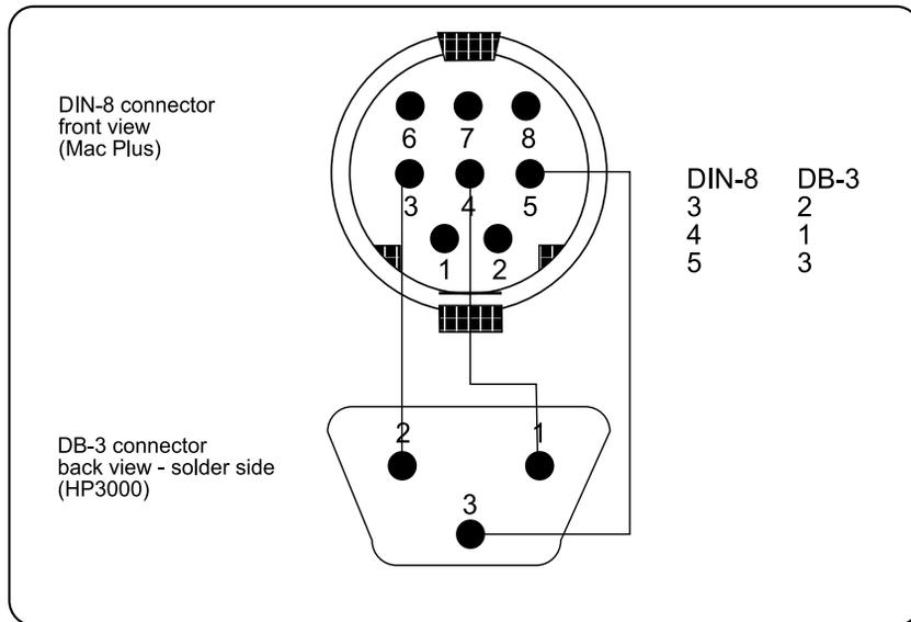
The above illustration shows a DIN-8 connector, front view (Mac Plus), and a DB-3 connector, back view - solder side (HP3000).
