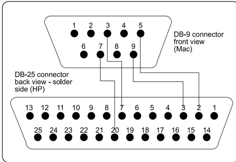
Connection of pin 7 on the DB-9 to pin 20 on the DB-25 is required only if you plan to use the Hardware DTR Hangup option in the *Connection Settings* box (choose *Connection* from the *Settings* menu). To use this option, you must have a 512KE or larger system.
