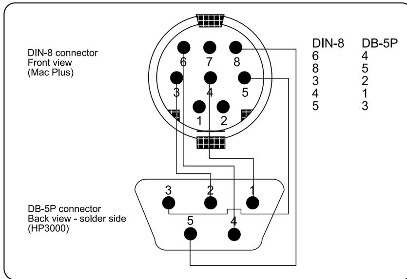
The above illustration shows a DIN-8 connector, front view (Mac Plus), and a DB-5P connector, back view - solder side (HP3000).
